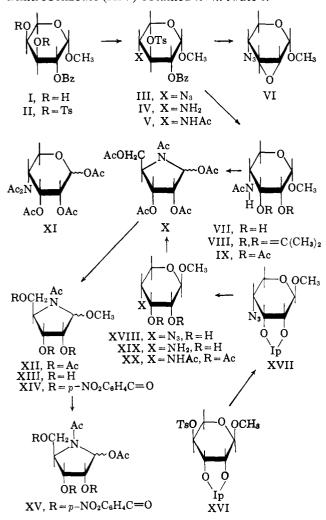
The contraction of the 4-acetamido-4-deoxyribopyranosides to the furanose ring under acid conditions is noteworthy. This is in direct contrast to the behavior of methyl 4-acetamido-2,3,6-tri-O-acetyl-4-deoxy- $\alpha$ -D-glucopyranoside which maintained the pyranose ring under these same conditions.<sup>11</sup> It is
